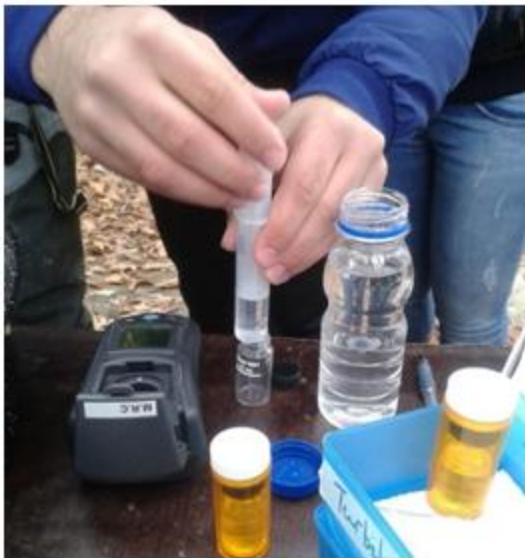
Image 10: Here the 10ml water is transferred in the bottle, after the team took a sample of water from the river. The bottle then goes into the turbid meter for measurements.
