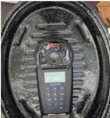
Image 14: Chrome meter - the measuring instrument that we used for the measurement of nutrients.
